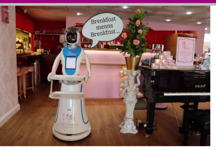
"If Theresa senses a person in its route, it will stop and then frown and ask the person to move out of its way before she continues on her way. This is part of the safety mechanism we developed for her with the robotics laboratory that manufactured Theresa for us in Japan," Shouly said, adding that Theresa uses laser-guided trackless navigation and ultra-sonic obstacle avoidance.
